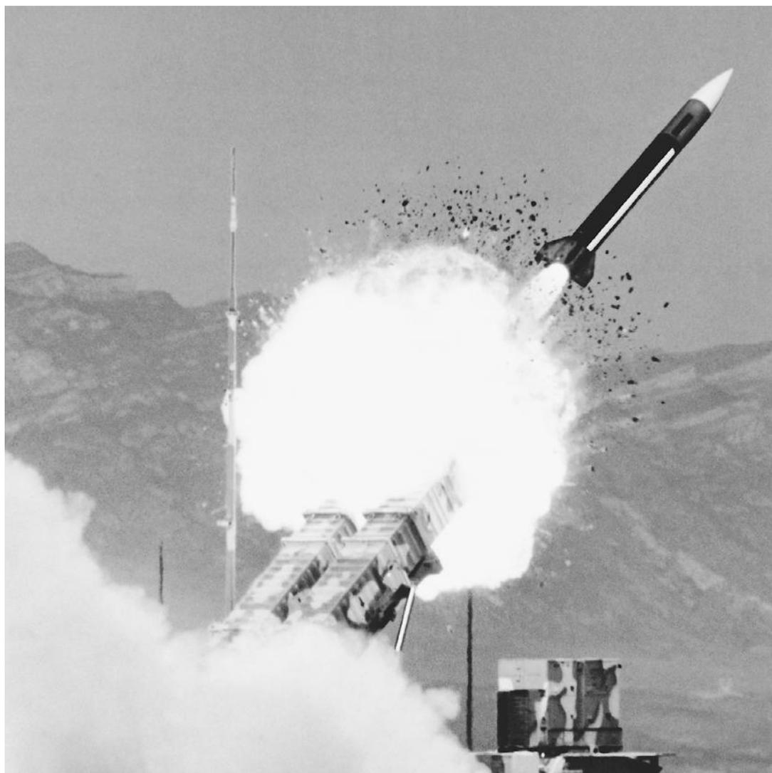
IN THE CASE OF A ROCKET, LIKE THIS PATRIOT MISSILE BEING LAUNCHED DURING A TEST, PROPULSION COMES BY EXPELLING FLUID—WHICH IN SCIENTIFIC TERMS CAN MEAN A GAS AS WELL AS A LIQUID—FROM ITS REAR END. MOST OFTEN THIS FLUID IS A MASS OF HOT GASES PRODUCED BY A CHEMICAL REACTION INSIDE THE ROCKET'S BODY, AND THIS BACKWARD MOTION CREATES AN EQUAL AND OPPOSITE REACTION FROM THE ATMOSPHERE, PROPELLING THE ROCKET FORWARD. (Corbis. Reproduced by permission.)
