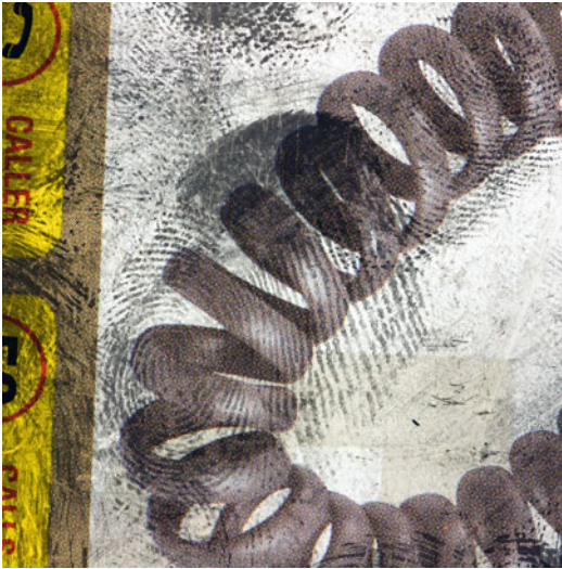
Fingerprint Identification, Fig. 2 Marks developed on a semi-porous printed cardboard box using black powder suspension
