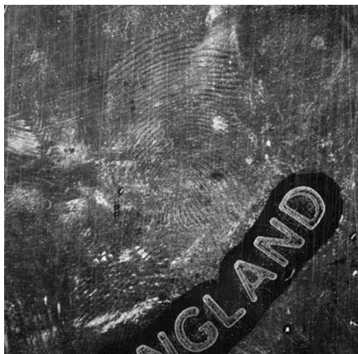
Fingerprint Identification, Fig. 1 A mark developed using aluminum flake powder and lifted using transparent tape
