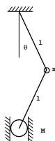
Figure 13.4 A model for a crane holding a heavy load, with an intermediate pulley in the cable. Doesn't the main load rise twice as much as the pulley?
