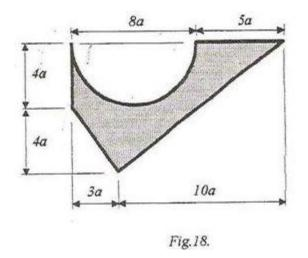
Problem 7. Determine the position of the centroid for the homogeneous plane plate
