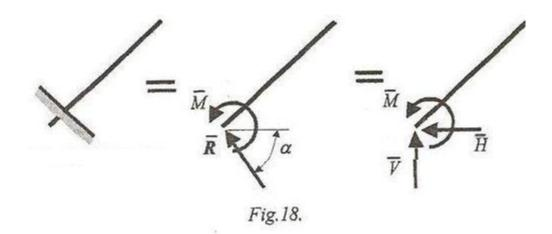
Being a non punctual constraint it will be replaced with a system of reaction forces. Reducing these forces in the theoretic point of fixation we have the force-couple system of the reactions made from two components: a reaction force having its magnitude and its direction unknowns and a moment reaction with unknown magnitude. For to simplify the using of this reactions we shall use two unknown reaction forces on two known directions and an unknown couple (moment).
