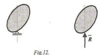
We remark that a simple support removes one degree of freedom and **introduces in calculation one scalar unknown as force**.
