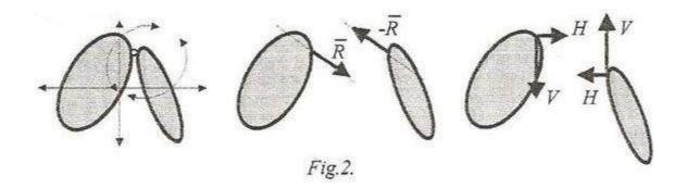
By definition the simple internal hinge is the ideal connection between two bodies that **fix a point of one body to a point of the other body**.
