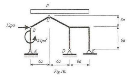
**Solution.** The system of bodies is made from three bodies (AB, BC, and CDE) and it is statically determined and stable:
