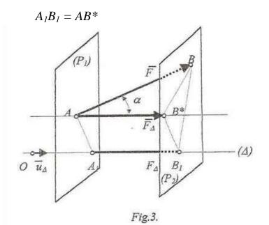
But this segment of line is the side of the right angle triangle ABB\* and it may be calculated resulting the expression of the projection of a force on the direction of an axis:
