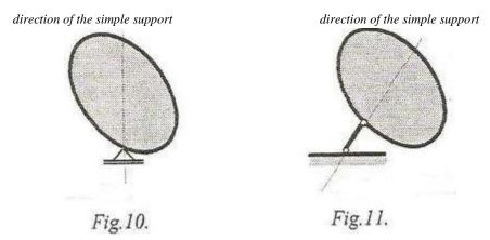
Using the axiom of constraints the simple support can be replaced with a reaction force having the following characteristics:
