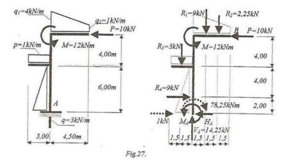
**Solution.** We shall make as in the previously problem. Firs we make the free body diagram replacing the fixed support with the three reactions (two forces and a concentrated moment) and the distributed force replaced with the corresponding resultant force.
