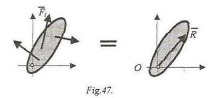
4)  $\overline{R} \neq 0$ ;  $\overline{M_0} \neq 0$  and  $\overline{R}$ .  $\overline{M_0} = 0$  namely the system of forces reduces to an **unique resultant force that does not pass through the point O**. In this case we have to determine the position of the unique resultant force that is the simplest equivalent system. The particular shape of the equation of the central axis in two dimensions (in plane) is:
