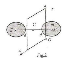
The masses of the two halves of the system (or of the body) are the same. Consequently we can calculate the statically moment about the symmetry plane:
