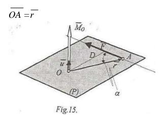
By definition, is called **moment of the force F with respect to the point O** the vector quantity, marked  $\overline{M}_0$  and equal to the vector product between the position vector of the point of application of the force with respect to the given point O and the force  $\overline{F}$ :
