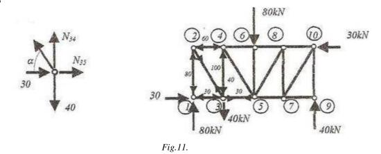
the internal forces which are represented on the scheme of the results as in the figure 11. The following joint is the joint 4.
