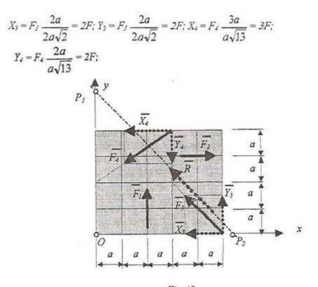
*Fig.49. The resultant force of the system of forces will have the projections on the two axes:*
