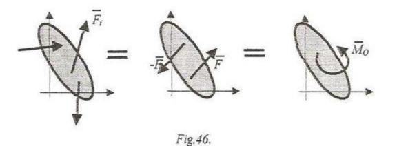
3)  $\overline{R} \neq 0$ ;  $\overline{M_0} = 0$ . In this case the simplest equivalent system is the unique resultant force passing through the point O.
