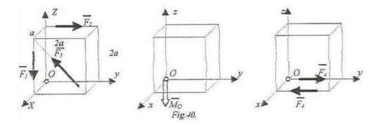
**Solution.** As in the previous problem first we shall decompose the forces in components parallel with the reference axes, in this way the force  $F_3$  will have two components:
