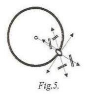
Results from these examples that there are constraints that remove one degree of freedom or two or more degrees of freedom. The constraints which remove one degree of freedom are called **simple constraints**, and those which remove more degrees of freedom are called **multiple constraints**.
