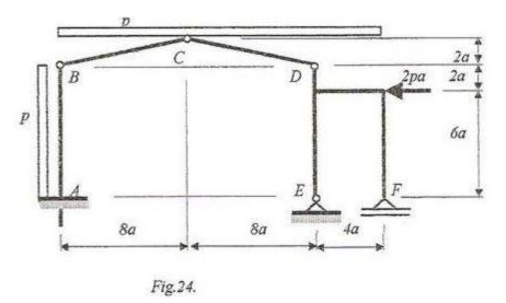
**Solution.** The system is made from four bodies and is statically determined and stable because it has one fixed support, four hinges and one simple support:
