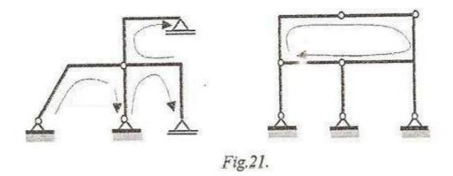
Supposing that the internal connections are only internal hinges, the systems with open outlines have the following two proprieties: 1) the number of the external unknowns is equal always with:
