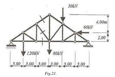
We shall number the joints in an any order and we shall calculate the sinuses and cosinuses of the angles  $\alpha$  and  $\beta$  that define the directions of the two members in which we shall calculate the internal forces.
