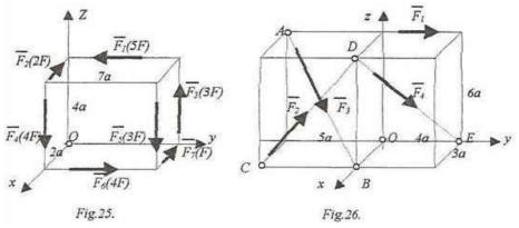
**Problem 10.** Calculate the resultant moment about the point O for the system of forces from the figure 26. Are known:  $F_1 = 4F$ ,  $F_2 = 2\sqrt{61}F$ ,  $F_3 = 3\sqrt{70}F$ ,  $F_4 = 3\sqrt{61}F$ .
