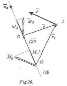
For to show that we may take any point from the axis about which is calculated the moment and the moment about the axis does not modify. We shall consider a point Q, from the axis, about which we have:
