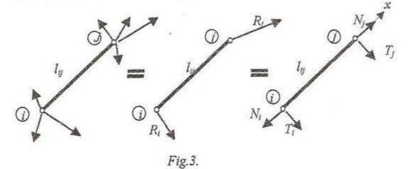
All the forces, given and reaction, will have the points of application in the two joints. Being concurrent forces they can be removed with their resultant forces acting in the two points. We decompose the two resultants in two components: one on the direction of the axis of the member ant the second on the normal direction on the member, marked respectively  $N_i$  and  $N_j$  and also  $T_i$  and  $T_j$ .
