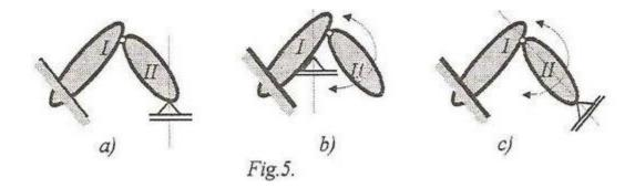
b) in figure 5.b. the system is not statically determined because the body II has not enough constraints for to be fixed (it has only one fixed hinge that cannot fixes the body, it has possibility to rotates about the hinge), but the body I has too much constraints for to by statically determined;
