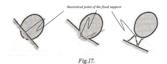
Because the bodies used in this part of the mechanics will be represented as bars this theoretical point of fixation is the intersection point between the axis of the rod and the surface of fixation. The scheme of this constraint is represented in the figure 18.
