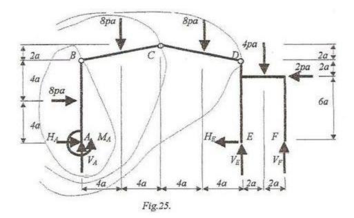
We shall write other three equations for the parts of the system and we shall choose that all the three equations for the same part namely the part that does not contain the body DEF (this body is taken as principal body for the previously three equations). We shall choose the left part of the system for to write these equations:
