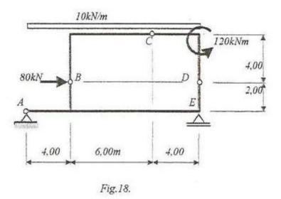
Solution. The system is statically determined and stable being made from three bodies having four hinges and one simple support and it is fixed because the body ABCD that is a principal body so it is fixed by its hinged support from A and simple support from E, and the part made from the bodies BC and CD (secondary part of the system) has two fixed hinges (in B and D) and an internal hinge in C (non collinear The free body diagram is obtained replacing only the external constraints, without to
