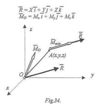
Suppose that in point A(x,y,z) the resultant moment is minimum, namely it is collinear with the resultant force. In the same time the resultant moment from this point may be expressed function of the components of the force –couple system in point O:
