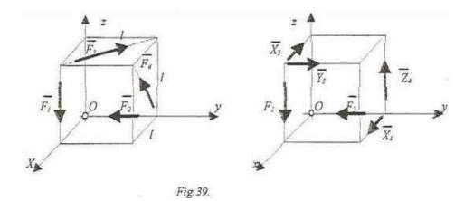
**Solution.** in the first step we shall decompose the forces of the system in components parallel with the reference axes. In this way the forces  $\overline{F_1}$  and  $\overline{F_2}$  are own components, the force  $\overline{F_3}$  has two components:  $\overline{X_3}$  and  $\overline{Y_3}$  and the force  $\overline{F_4}$  will have also two components  $\overline{X_4}$  and  $\overline{Z_4}$ . These components will have the following magnitudes:
