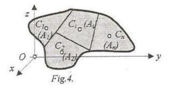
We shall consider the plate divided into simple plates for which we know the areas and the positions of the centroides. The  $x_c$  coordinate of the centroid of the whole plate is calculated:
