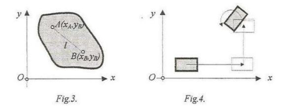
If we want to change the position of the body we have three independent possibilities of motion (two translations parallel to the axes of a
