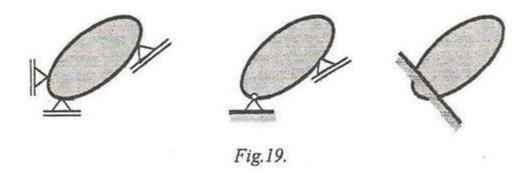
Finally the body may be fixed with **one fixed support** that introduces in equations three unknowns.
