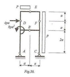
**Solution.** We remark that the system is symmetrical but the load is an any load, consequently if we want to use the proprieties of the symmetrical systems we need to divide the load in the two components: one symmetrical and one antisymmetrical.
