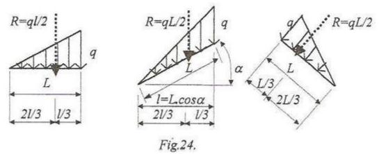
• **Trapezoidal distributed force**. This load is a system of forces distributed linearly as the triangular distribution but the first value is not zero. The simplest way to work with this force is that to consider a superposition (an addition) of two triangular forces: one with the maximum value  $q_1$  and the second with the maximum value  $q_2$  and with the same length of distribution.
