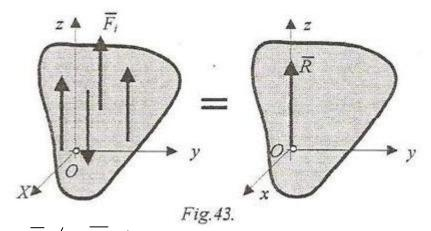
• 4)  $\overline{R} \neq 0$ ,  $\overline{M_0} \neq 0$ , and  $\overline{R}$ .  $\overline{M_0} = 0$ . In this case the system is reduced to an unique resultant force that does not passé through the point O. Consequently we have to determine the position of this force using the equation of the central axis. This equation becomes for the parallel forces with the Oz axis:
