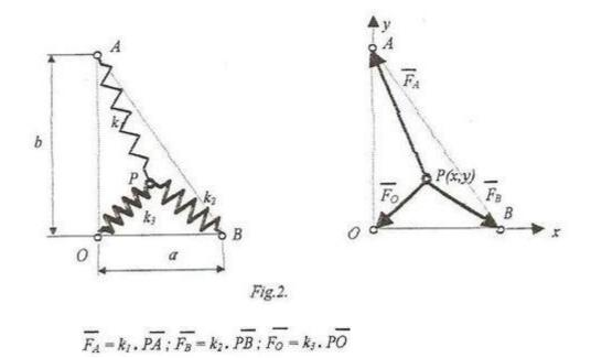
The equilibrium equations of the particle P are obtained projecting the three forces on the two axes of the reference system. At calculation of these projections we will consider that in fact we project the position vectors of the three points O, A and B with respect to the point P. We have:
