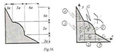
**Solution.** We remark that the plate is symmetrical having as symmetry axis the bisecting line of the 90° angle. After which we divide the body in five simple plates(two rectangles, two right angle triangles and one quarter of circle) we shall choose as system of reference the system having the origin on the symmetry axis and passing through the centers of the two triangles. This system will make to have:
