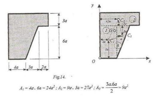
Step 2. The reference system will be taken such as the entire plate to be located in the first frame. In this way all the coordinates will be positive.
