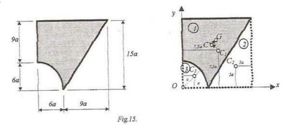
**Solution.** We shall choose as option of division of this plate to subtract a triangle and a quarter of circle from the square with 15a as side. As system of reference we shall choose the system having the axes tangent to the body, in this way the body will be located in the first frame.
