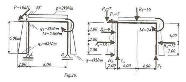
**Solution. Step 1.** The body is statically determined and stable because it has a hinge and a simple support, and the direction of the simple support doesn't pass through the hinge.
