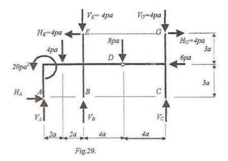
This part is also a system with open outlines and consequently we shall solve in the same way as the secondary part using the mixed method. The equilibrium equations will be:
