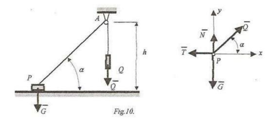
**Solution.** The particle has only one constraint with friction (the horizontal rough surface) because the string is not a constraint. Having one single constraint the particle has one degree of freedom, so it has one possibility of motion to slide on the horizontal plane. Because the force Q the particle has the tendency to move on the right sense.
