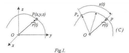
Because the particle is in motion (changes its potion in time) the position vector is a function of time:
