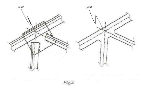
We make the remark that the external constraints are considered located in the joints also.
