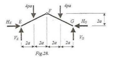
This part is a system with open outlines and so we can solve using the mixed method for to determine the four unknowns. We shall make the remark that the equations for the entire subsystem are in fact equations for a part of the entire initial system. The equilibrium equations will be:
