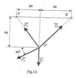
**Problem 4.** Calculate and represent the resultant force of the following system of concurrent forces knowing the magnitudes :  $F_1 = 5F$ ,  $F_2 = 3\sqrt{41}F$ ,  $F_3 = 4\sqrt{13}F$ ,  $F_4 = 3\sqrt{14}F$ .
