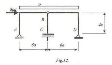
**Solution.** The system is made from three bodies and has a fixed support, two simple hinges and one double hinge (this hinge makes the connection between three bodies) in B. Therefore it is statically determined:
