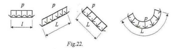
Being a system of forces, the uniformly distributed force can be replaced with a resultant force having as magnitude the product between the intensity of it and the length of distribution:
