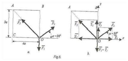
**Solution. Step 1.** First we shall remark that the system of forces is also a coplanar one, namely the forces of the system are located in the same plane. Consequently, we shall choose as reference system the plane system Oxy with the origin in the common point of application of the forces.
