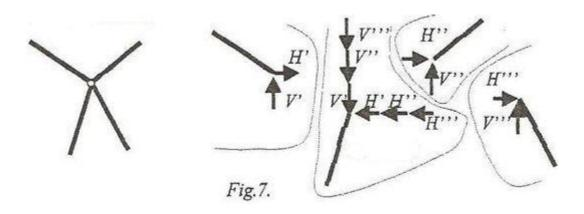
The resulted scheme is the **free body diagram** corresponding to this method.
