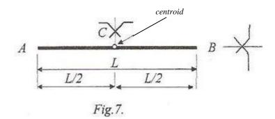
Because the bar has a symmetry point in the middle of the length of the rods, in that point is located the centroid of it. Namely the centroid of a rectilinear bar is located in the middle of the distance between the ends of the bar.
