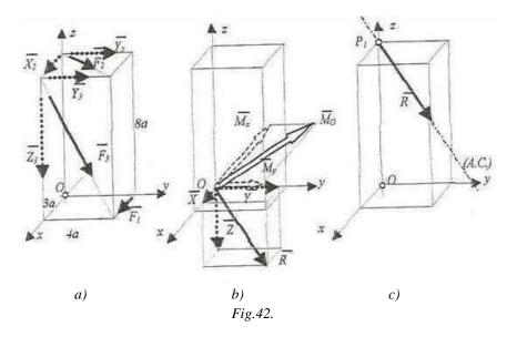
**Solution.** First we shall decompose the forces  $\overline{F_2}$  and  $\overline{F_3}$  in two components having the
