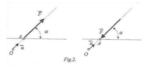
The magnitude of the force is defined, using the units of measure of the force, by a scalar quantity. The magnitude is represented using an any scale (the correspondence between the units of the force and the unites of the length) through a segment of line.
