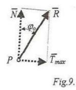
To consider now the limit state of the particle when the friction force has its maximum value. We mark  $\varphi_o$  the angle made among the ideal reaction force and the real reaction force. This angle is called **maximum** friction angle. The tangent of this angle may be expressed from one right angle triangle:
