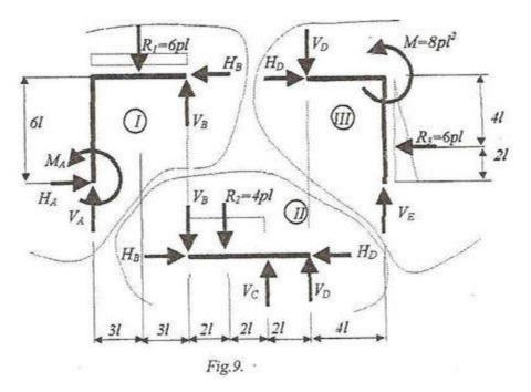
Step 3. For each body we shall write three equilibrium equations, namely: for the body I, that has a fixed support, we shall prefer two projections and a moment equation about the fixed support, and for the other two bodies we prefer two moment equations and one projection. The equations will be: -for the body I:
