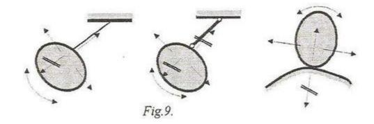
cases is removed the possibility of motion on the direction of the string, or of the rod, or of the normal direction on the tangent in the point of support. In this way the simple support removes, always, **one degree of freedom**. The other two possibilities of motion are free (here the translation on the normal direction and the rotation).
