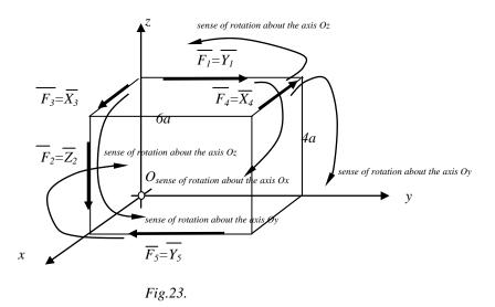
The distance from the axis Ox to the support line of the force is perpendicular on the both directions (of the axis and of the support line of the force). If the body is a parallelipipedium, like in this problem, then the distance is the side perpendicular on the both directions, here the side  $l_z$ .
