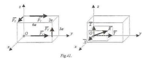
**Solution.** Because the forces of the system are parallel to the reference axes we shall calculate the force-couple system in point O. Are obtained the projections of the resultant force:
