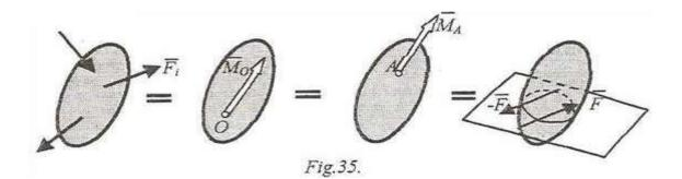
• 3)  $R \neq 0$ ;  $\overline{M_0} = 0$ . The force-couple system in point O has a single component namely the resultant force. In the same time the force couple system is an equivalent system for the given system of forces, so the resultant force is the simplest equivalent system. We shall say that the system of forces is reduced to a unique resultant force that pass through the point O.
