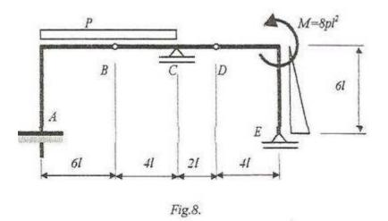
**Solution. Step 1.** The system of bodies is made from three bodies, has a fixed support in A, two simple supports in C and E and two internal simple hinges in B and D. The quantitative condition of statically determination is:
