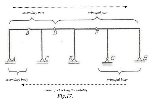
support is also a fixed one). This part has in its constraints and connections eight scalar unknowns (two in D, two in F and two in G and one unknown in E and in H).
