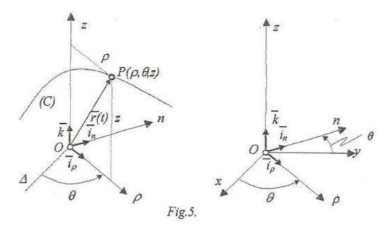
But to define the position of the particle in space is necessary to define the position of the reference system with respect to another fixed system. This fact is made if it is known the angle  $\theta$  measured between a fixed plane from space (for example the  $\Delta Oz$  plane) and the moving plane  $\rho Oz$ . Results that the position of the particle in scalar way is given by three coordinates:
