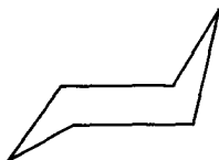
Fig. 264. Chair configuration of S_6 rings in \rho -sulphur.
