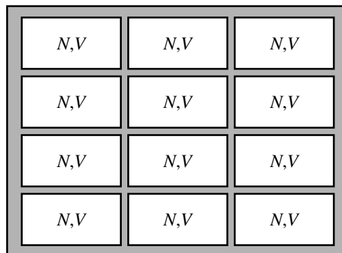
Figure 16.3 Canonical ensemble of systems each having the same N and V . The canonical ensemble contains \eta systems, isolated from one another after having been in contact with a heat reservoir at temperature T .
