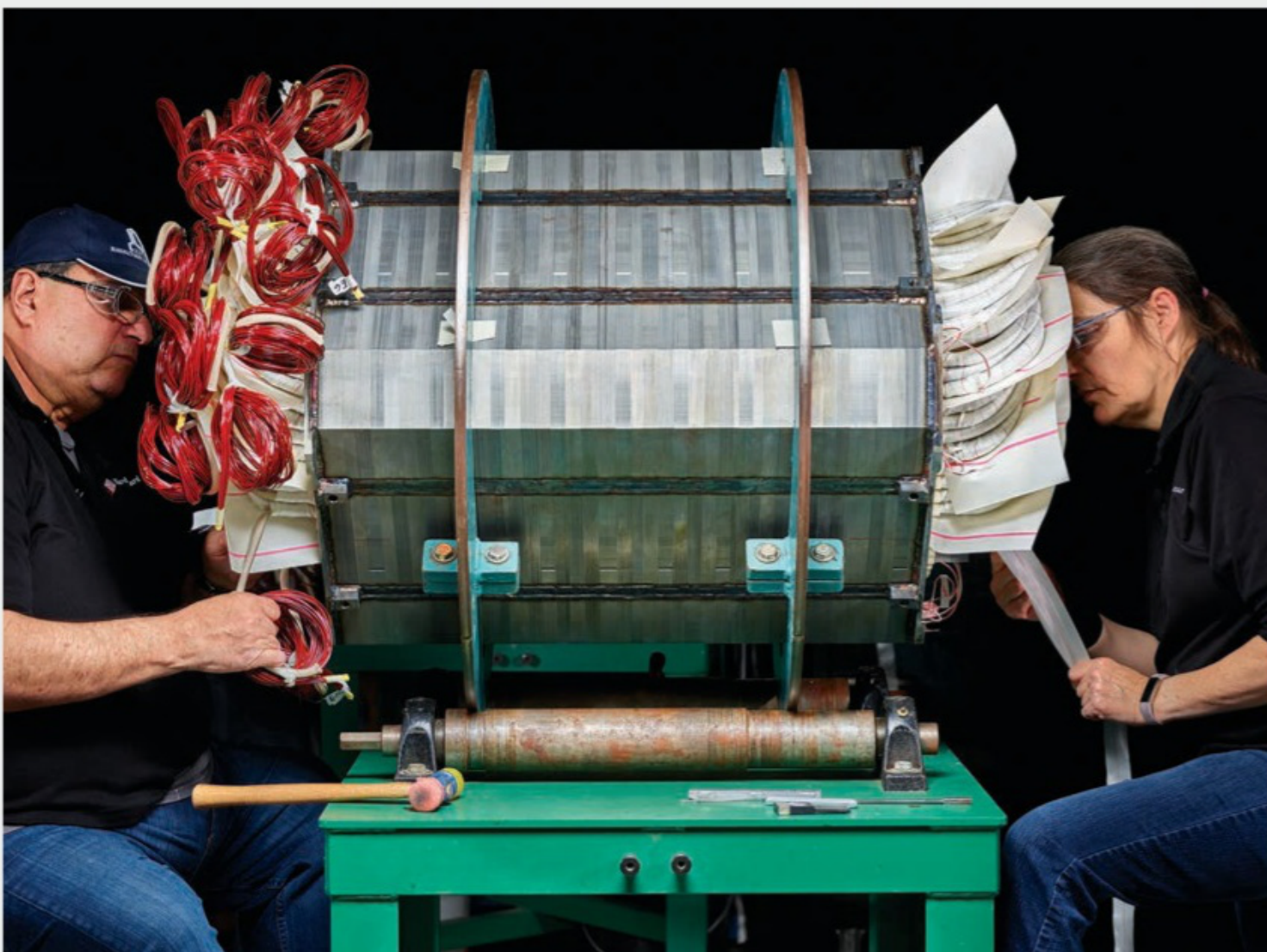
Making motors by hand enables a level of customization that is important to Ward Leonard customers such as the United States Navy, whose ships rely on motors that can weather harsh conditions.
