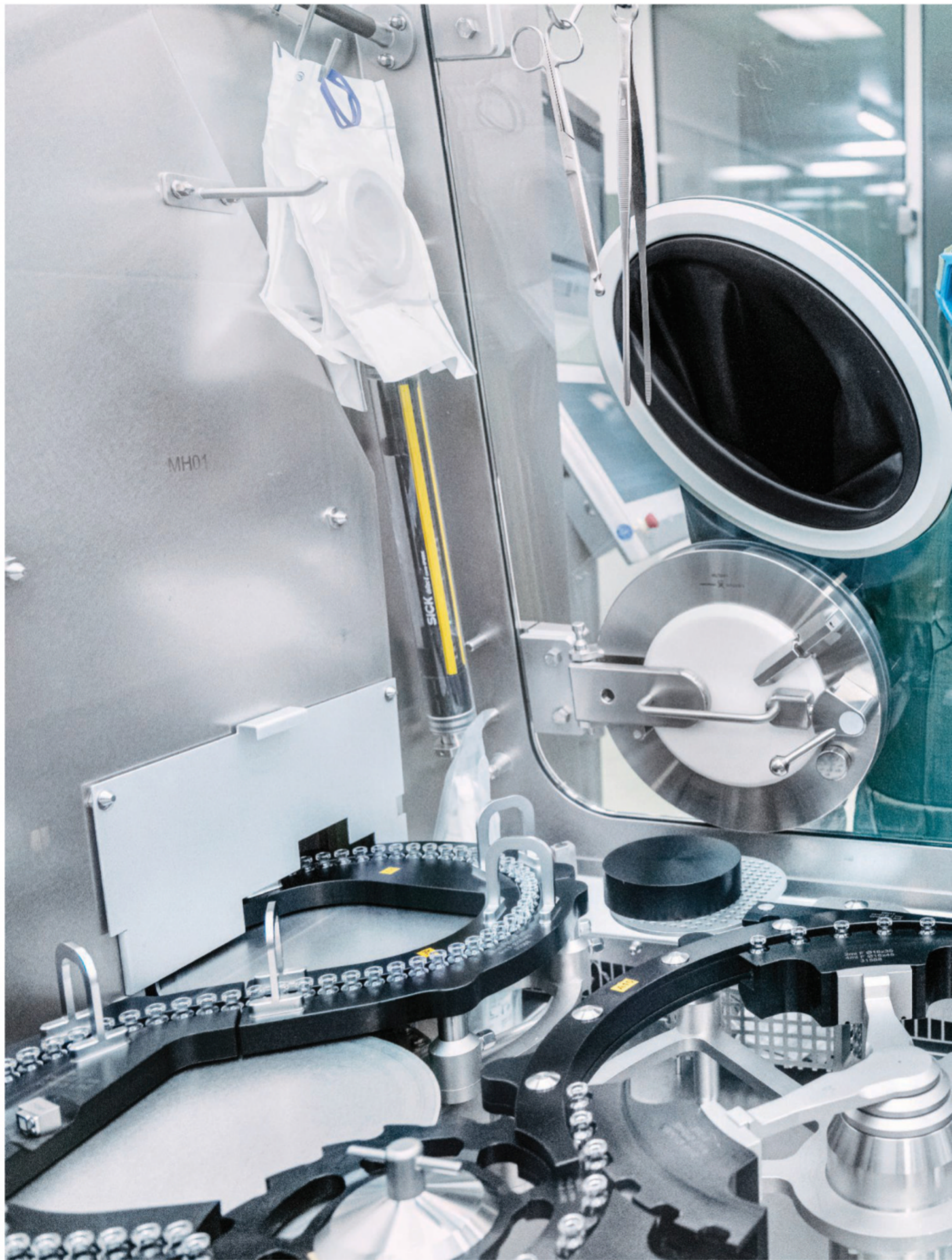
At the fill-and-finish facility operated by Baxter International in Halle, 120 miles north of Marburg, technicians monitor the washing and sterilization of the vials before they are filled with vaccine, then stoppered and sealed
