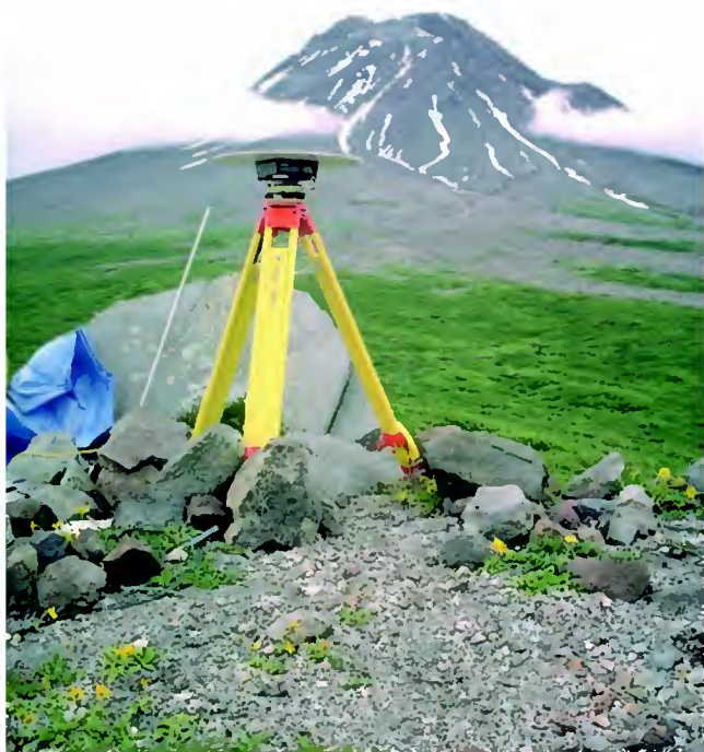
Figure 2.30 Using GPS to measure landscape change. Given the high accuracy of some GPS systems, it is possible to monitor changes in ground elevation, such as those that may occur near the Augustine Volcano in Alaska due to renewed volcanic activity.
