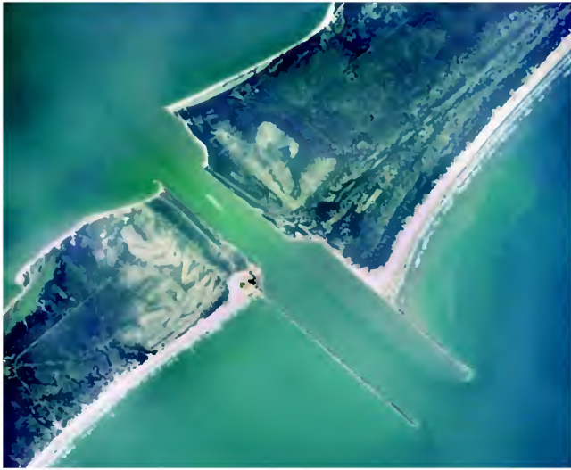
Figure 19.40 A typical jetty. This jetty on the Texas coast provides a reliable passageway into the ocean for boats. Given the variable beach thickness on either side of the jetty, can you tell which way the longshore current is flowing? Note the sequence of foredunes on the updrift (arrow) side of the jetty. These dunes formed due to high sand supply because sand was trapped.
