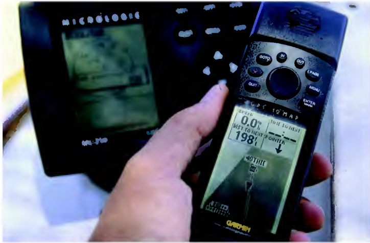
Figure 2.28 A hand-held GPS receiver. This unit receives the PRC signal from satellites in the GPS constellation.
