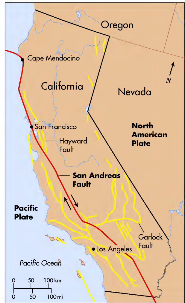
Figure 13.24 California fault systems. The San Andreas Fault is a transform fault that forms the boundary between the North American (to the east) and Pacific (to the west) plates. Arrows on either side of the fault reflect the relative movement of plates. Note the various subsidiary faults in the system.
