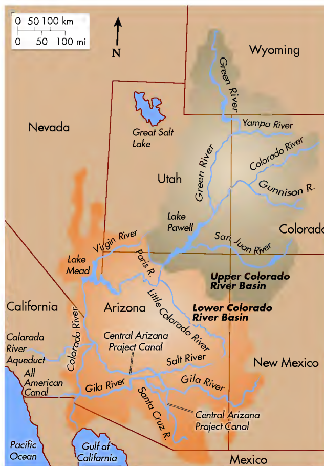
Figure 20.7 Regulation of water in the Colorado River basin. The Colorado River Compact divided the watershed into an upper and lower basin. Water in each of these basins is strictly regulated, with a set amount allowed for each region. The Central Arizona Project and Colorado River Aqueduct divert water from the Colorado River to southern Arizona and southern California, respectively, for human purposes.
