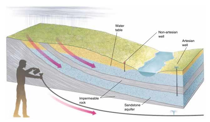
**Figure 15–7** An artesian aquifer forms where a tilted layer of permeable rock, such as sandstone, lies sandwiched between layers of impermeable rock, such as shale. Water rises in an artesian well without being pumped. A hose with a hole shows why an artesian well flows spontaneously.
