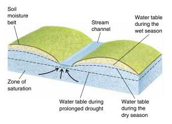
**Figure 15–4** The water table follows topography, rising beneath a hill and sinking beneath a valley. Dashed lines show that it also sinks during drought and rises during the rainy season. The arrows show ground-water flow.
