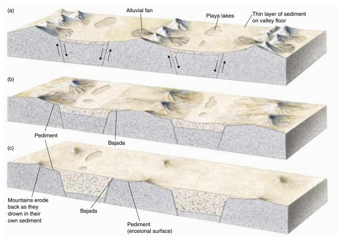
**Figure 16–12** One scenario for the formation of bajadas and pediments. (a) The mountains and valleys were formed by block faulting. Desert streams deposit sediment to form alluvial fans. (b) Alluvial fans merge, creating a broad undulating surface called a bajada. (c) The mountain range erodes backward, creating a pediment along the mountain front.
