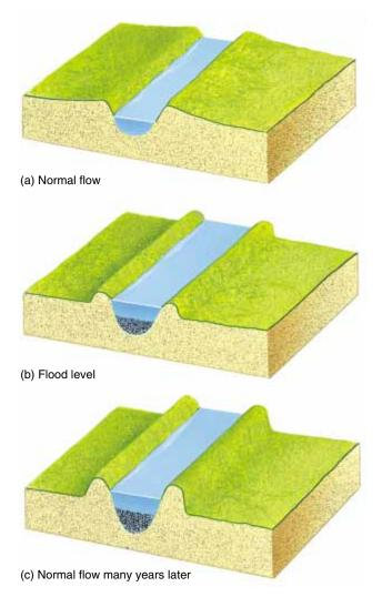
**Figure 14–30** Artificial levees cause sediment to accumulate in a stream channel, eventually raising the channel above the level of the flood plain and creating the potential for a disastrous flood.
