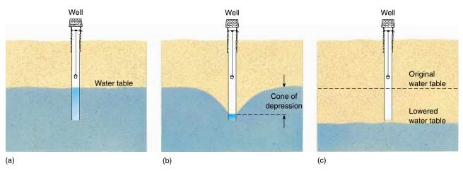
**Figure 15–8** (a) A well is drilled into an aquifer. (b) A cone of depression forms because a pump draws water faster than the aquifer can recharge the well. (c) If the pump continues to extract water at the same rate, the water table falls.
