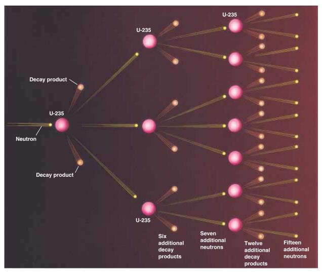
**Figure 19–23** When a neutron strikes a uranium-235 nucleus, the nucleus splits into two roughly equal fragments and emits two or three neutrons. These neutrons can then initiate additional reactions, which produce more neutrons. A branching chain reaction accelerates rapidly through a sample of concentrated uranium-235.
