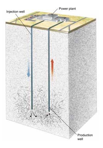
**Figure 15–23** A schematic view of the Fenton Hill, New Mexico, dry geothermal energy plant.
