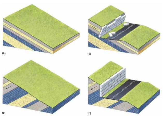
**Figure 13–2** (a) Sedimentary rock layers dip parallel to this slope. (b) If a road cut undermines the slope, the dipping rock provides a good sliding surface, and the slope may fail. (c) Sedimentary rock layers dip at an angle to this slope. (d) The slope may remain stable even if it is undermined.
