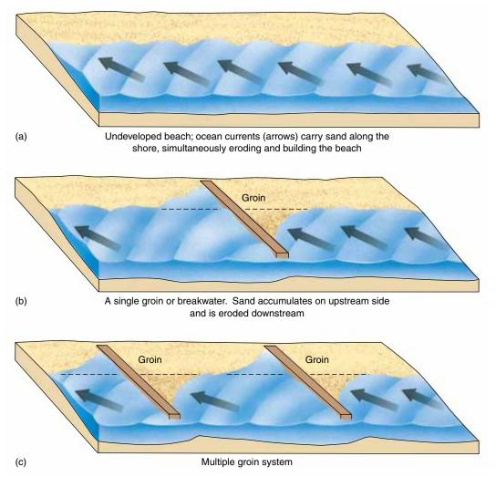
**Figure 18–21** (a) Longshore currents simultaneously erode and deposit sand along an undeveloped beach. (b) A single groin or breakwater traps sand on the upstream side, resulting in erosion on the downstream side. (c) A multiple groin system propagates the uneven distribution of sand along the entire beach.
