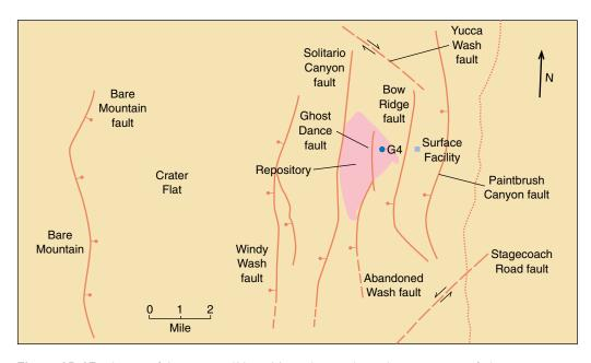
**Figure 15–17** A map of the proposed Yucca Mountain repository shows numerous faults where rock has fractured and moved during the past 2 million years. (Redrawn from *Geotimes*, January 1989)
