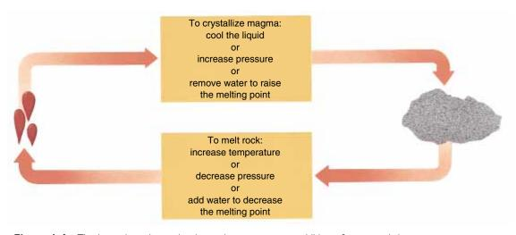
**Figure 4–6** The lower box shows that increasing temperature, addition of water, and decreasing pressure all melt rock to form magma. The upper box shows that cooling, increasing pressure, and water loss all solidify magma to form an igneous rock.
