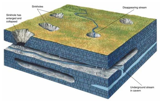
**Figure 15–19** Sinkholes and caverns form in limestone. Streams commonly disappear into sinkholes and flow through the caverns to emerge elsewhere.
