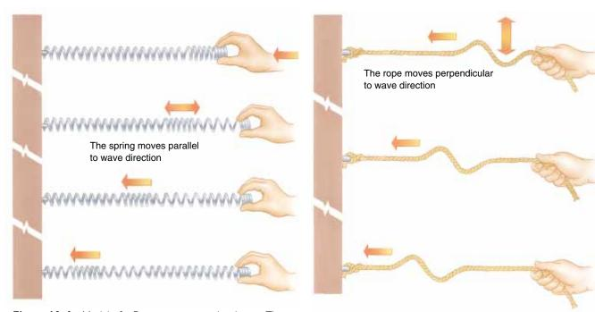
**Figure 10–6** Model of a P wave; a compressional wave. The wave is propagated along the spring. The particles in the spring move parallel to the direction of wave propagation.
