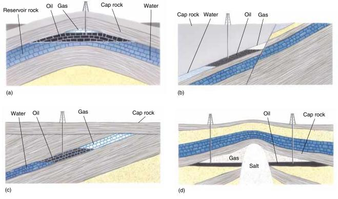
**Figure 19–19** Four different types of oil traps. (a) Petroleum rises into permeable limestone in a structural dome. (b) A trap forms where a fault has moved impermeable shale against permeable sandstone. (c) Horizontally bedded shale traps oil in tilted limestone. (d) In a salt dome, a sedimentary salt deposit rises and deforms overlying strata to create a trap.
