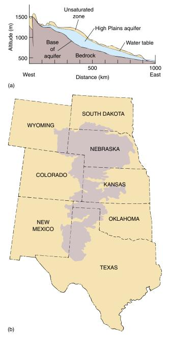
**Figure 15–10** The Ogallala aquifer supplies water to much of the High Plains. (a) A cross-sectional view of the aquifer shows that much of its water originates in the Rocky Mountains and flows slowly as ground water beneath the High Plains. (b) A map showing the extent of the aquifer.
