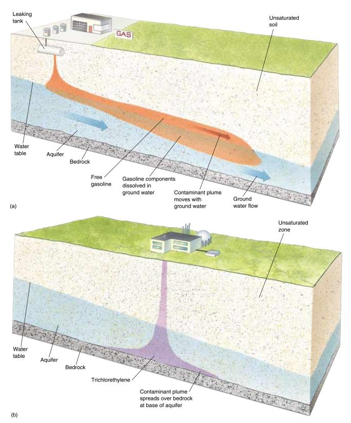
**Figure 15–14** (a) Gasoline and many other contaminants are lighter than water. As a result, they float and spread on top of the water table. Soluble components may dissolve and migrate with the ground water. (b) Other pollutants, such as trichlorethylene, are heavier than water and may sink to the base of an aquifer.
