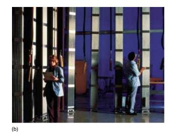
**Figure 19–24** (a) Fuel pellets containing enriched uranium-235. Each pellet contains the energy equivalent of I ton of coal. (b) Fuel pellets are encased into narrow rods that are bundled together and lowered into the reactor core. (Courtesy Westinghouse Electric Corp, Commercial Nuclear Fuel Division)
