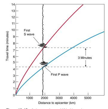
**Figure 10–13** A time-travel curve. With this graph you can calculate the distance from a seismic station to the source of an earthquake. In the example shown, a 3-minute delay between the first arrivals of P waves and S waves corresponds to an earthquake with an epicenter 1900 kilometers from the seismic station.
