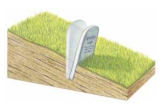
Figure 13–7 During creep, the soil surface moves more rapidly than deeper layers, so the tombstone embedded in the soil tilts downhill.
