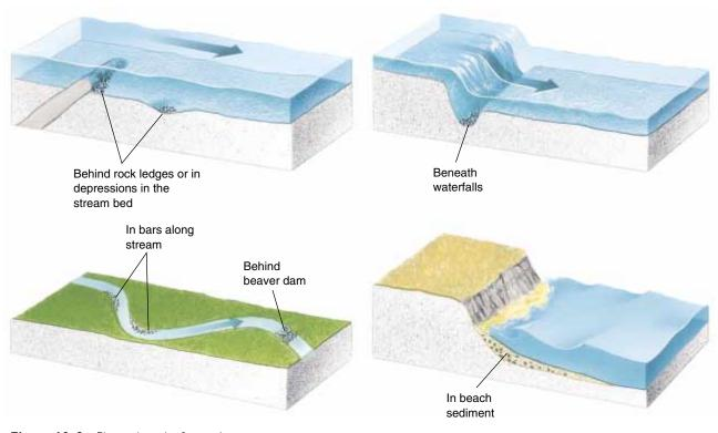
Figure 19–8 Placer deposits form where water currents slow down and deposit heavy minerals.
