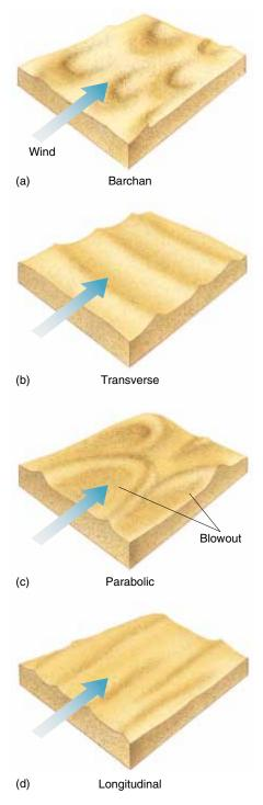
**Figure 16–22** Sand dunes take on different shapes depending on sand supply and variations in wind direction. (a) Barchan dunes. (b) Transverse dunes. (c) Parabolic dunes. (d) Longitudinal dunes.
