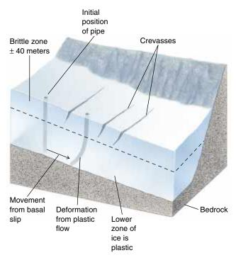
**Figure 17–5** In this experiment, a pipe is driven through a glacier until it reaches bedrock. The entire pipe moves downslope. The pipe becomes curved because the center of the glacier deforms plastically and moves faster than the base. The top 40 meters of ice are brittle, and the pipe remains straight in this section.
