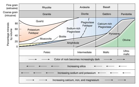
**Figure 4–16** The names of common igneous rocks are based on the minerals and texture of a rock. In this figure, a mineral's abundance in a rock is proportional to the thickness of its colored band beneath the rock name. If a rock has a fine grain texture, its name is found in the top row of rock names; if it has a coarse grain texture, its name is in the second row.
