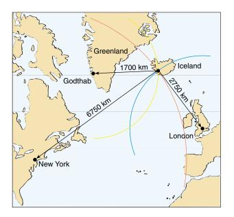
**Figure 10–14** Locating an earthquake. The distance from each of three seismic stations to the earthquake is determined from time-travel curves. The three arcs are drawn. They intersect at only one point, which is the epicenter of the earthquake.
