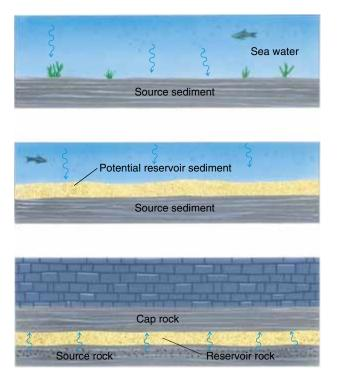
Figure 19–18 Most oil forms in shaly source rock. It must migrate to a permeable reservoir in order to be recovered from an oil well.
