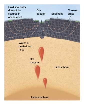
Figure 19–6 Submarine hydrothermal ore deposits precipitate from circulating seawater near the mid-oceanic ridge.
