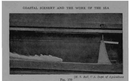
A suspension current of muddy water approaching the dam in a laboratory tank
