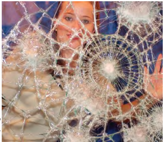
Figure 14-20. Fracture patterns on tempered glass.
