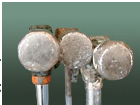
Figure 16-6. Unique markings such as nicks and ridge marks can be seen on the striking surface of three hammers.
