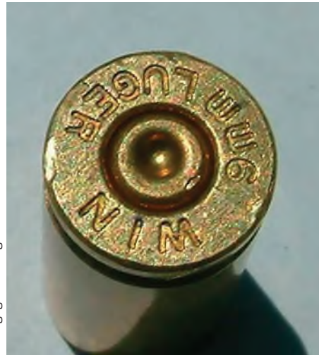
Figure 17-8. Ammunition has a headstamp—either a logo or name identifying the caliber and manufacturer. The headstamp is located on the bottom of the cartridge casing. Shown is the headstamp of a Luger 9mm.
