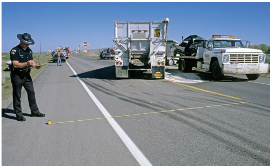
Figure 15-14. In a multiple-car accident, skid marks are used to determine the path and speed of each vehicle.
