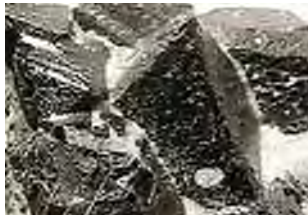
b. Magnetite is opaque black or gray. It is a form of iron oxide.
