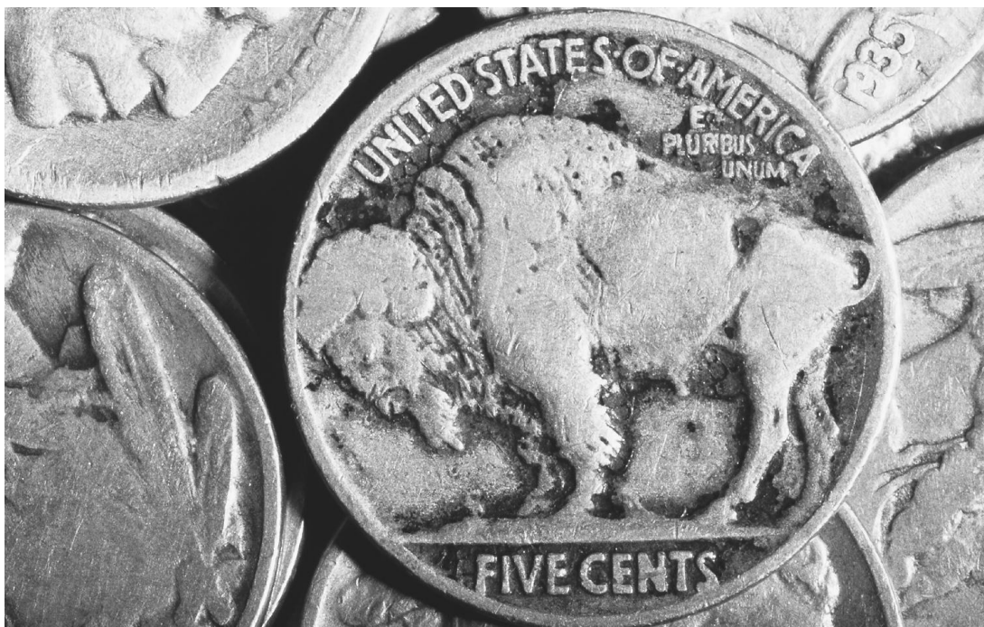
THE AMERICAN FIVE-CENT COIN, CALLED A “NICKEL,” IS ACTUALLY AN ALLOY OF NICKEL AND COPPER. (Layne Kennedy/Corbis. Reproduced by permission.)
