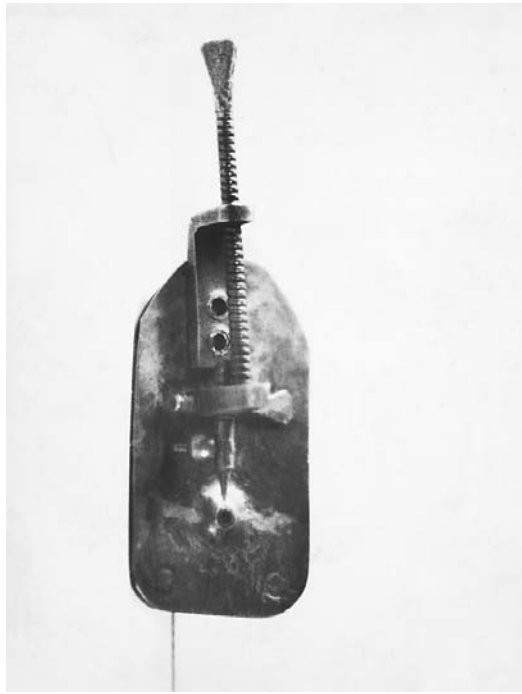
ANTON VAN LEEUWENHOEK'S PROTOTYPE MICROSCOPE. THE INVENTION OF THE MICROSCOPE MADE IT POSSIBLE TO SEE BACTERIA AND OTHER MICROORGANISMS, WHICH VAN LEEUWENHOEK, THE FIRST HUMAN BEING TO OBSERVE THEM, DUBBED ANIMALCULES, OR "TINY ANIMALS." (© Bettmann/Corbis. Reproduced by permission.)
