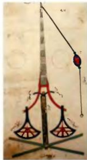
A traction trebuchet for hurling missiles from a 14 th -century Manual on Armoury by Ibn Aranbugha al-Zardkash.
