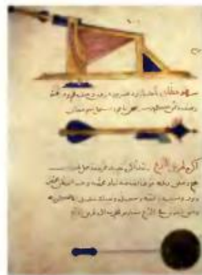
Cannon with adjustable mounting from a 14 th -century Manual on Armoury by Ibn Aranbugha al-Zardkash.
