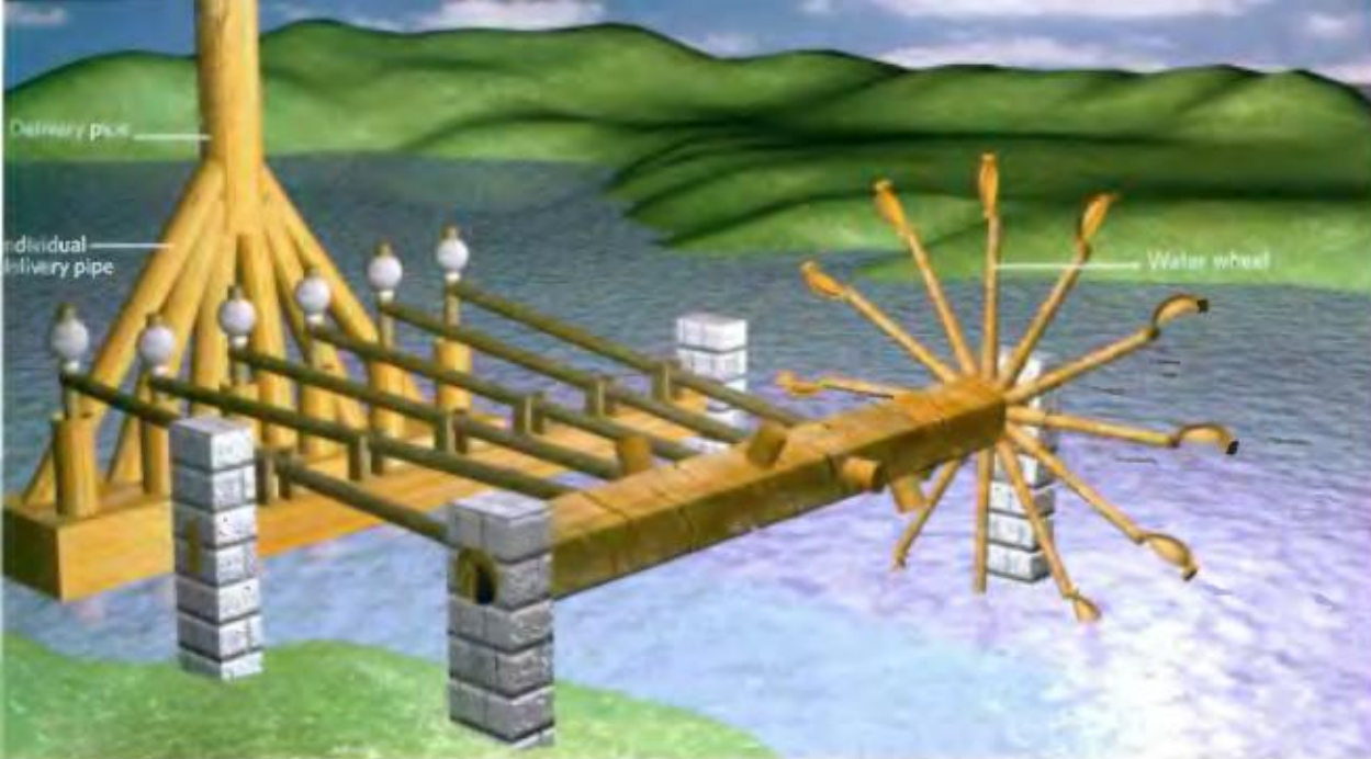
Above: Taqi al-Din's six-cylinder water pump. Note the cam shaft controlling the motion of the connecting rods to produce a progressive motion of the six pistons, so that water is raised continuously.
