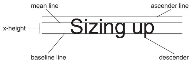
**Figure 5.1** Elements of a typeface
