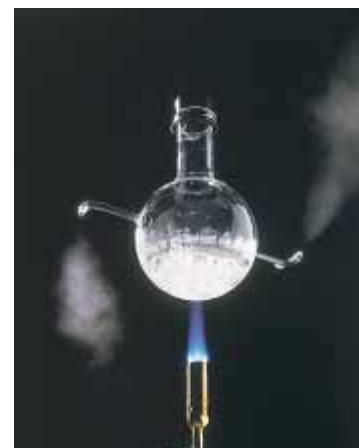
This device, called Hero's engine , was invented around 150 B.C. by Hero in Alexandria. When water is boiled in the flask, which is suspended by a cord, steam exits through two tubes at the sides (in opposite directions), creating a torque that rotates the flask.
