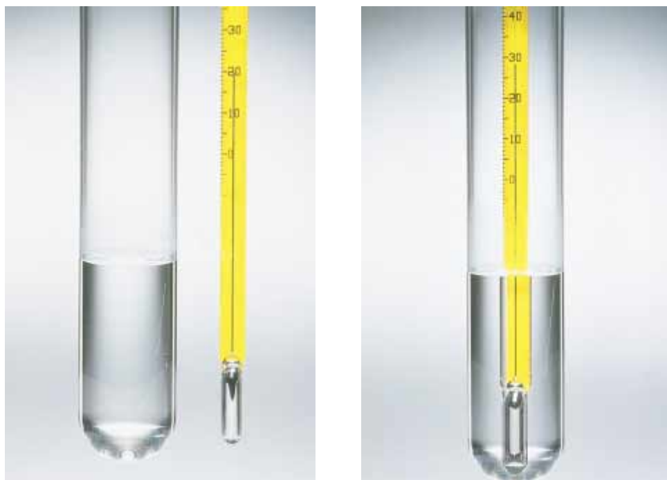
Figure 19.1 As a result of thermal expansion, the level of the mercury in the thermometer rises as the mercury is heated by water in the test tube.
