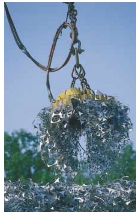
An electromagnet is used to move tons of scrap metal.
