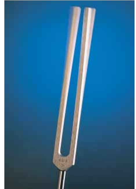
The sound from a tuning fork is produced by the vibrations of each of its prongs.
