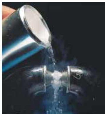
Oxygen, a paramagnetic substance, is attracted to a magnetic field. The liquid oxygen in this photograph is suspended between the poles of the magnet.
