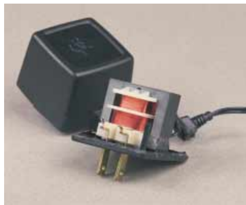
Figure 33.20 The primary winding in this transformer is directly attached to the prongs of the plug. The secondary winding is connected to the wire on the right, which runs to an electronic device. Many of these power-supply transformers also convert alternating current to direct current. (George Semple)
