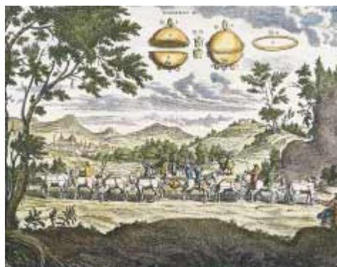
Figure P15.58 The colored engraving, dated 1672, illustrates Otto von Guericke’s demonstration of the force due to air pressure as performed before Emperor Ferdinand III in 1657. (
