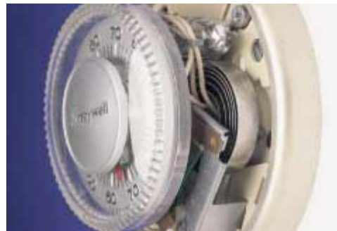
Figure 19.9 (a) A bimetallic strip bends as the temperature changes because the two metals have different expansion coefficients. (b) A bimetallic strip used in a thermostat to break or make electrical contact. (c) The interior of a thermostat, showing the coiled bimetallic strip. Why do you suppose the strip is coiled?
