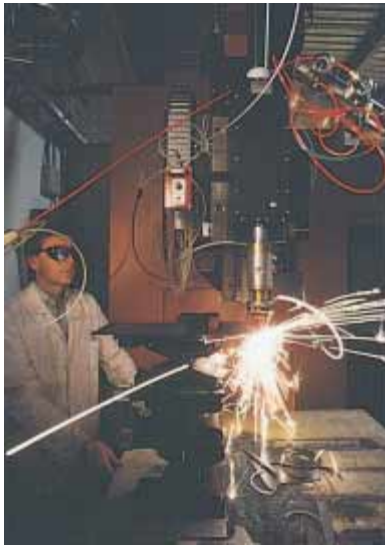
Figure P34.21 A laser cutting device mounted on a robot arm is being used to cut through a metallic plate. (Philippe Plailly/SPL/Photo Researchers)
