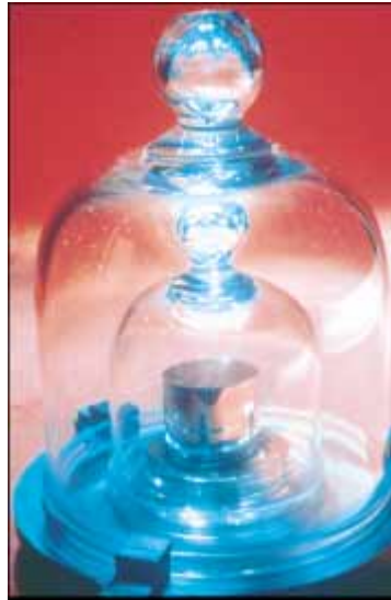
Figure 1.1 (Top) The National Standard Kilogram No. 20, an accurate copy of the International Standard Kilogram kept at Sèvres, France, is housed under a double bell jar in a vault at the National Institute of Standards and Technology (NIST). (Bottom) The primary frequency standard (an atomic clock) at the NIST. This device keeps time with an accuracy of about 3 millionths of a second per year. (Courtesy of National Institute of Standards and Technology, U.S. Department of Commerce)
