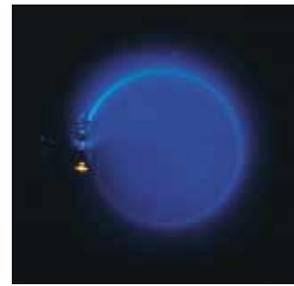
Figure 29.19 The bending of an electron beam in a magnetic field.
