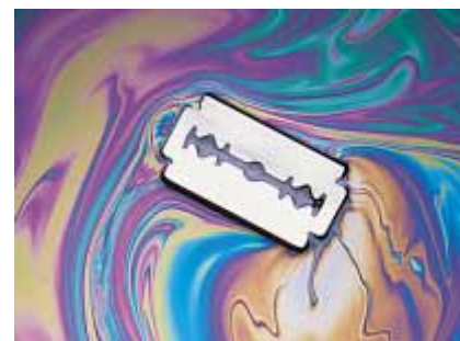
Figure 37.17 A thin film of oil floating on water displays interference, as shown by the pattern of colors produced when white light is incident on the film. Variations in film thickness produce the interesting color pattern. The razor blade gives one an idea of the size of the colored bands.
