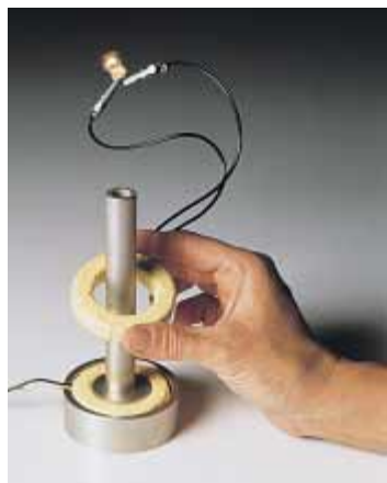
A demonstration of electromagnetic induction. A changing potential difference is applied to the lower coil. An emf is induced in the upper coil as indicated by the illuminated lamp. What happens to the lamp's intensity as the upper coil is moved over the vertical tube? (Courtesy of Central Scientific Company)
