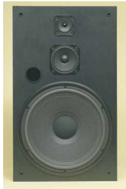
Figure 38.16 An audio speaker system for high-fidelity sound reproduction. The tweeter is at the top, the midrange speaker is in the middle, and the woofer is at the bottom. (International Stock Photography)
