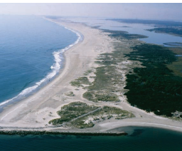
FIGURE 5.18 A barrier island, Assateague, along the Maryland-Virginia coast. Grasses cover and protect dunes, which keep ocean waves from disturbing the bay, salt marshes, and coast at right. Roads cut through the dunes expose them to erosion.
