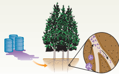
Plants can absorb, concentrate, and even decompose toxic contaminants in soil and groundwater.
