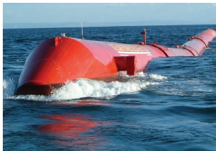
FIGURE 20.33 The Pelamis wave converter (named after a sea snake) is a 125 m long and 3.5 m diameter tube-hinged, so it undulates as ocean swells pass along it. This motion drives pistons that turn electrical generators. Energy experts calculate that capturing just 1 to 2 percent of global wave power could supply at least 16 percent of the world's electrical demand.
