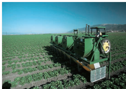
FIGURE 10.30 This machine, nicknamed the "sallad vac," vacuums bugs off crops as an alternative to treating them with toxic chemicals.
