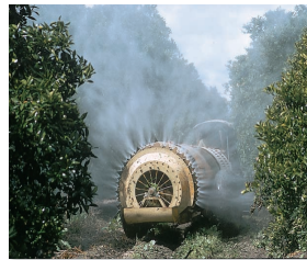
FIGURE 10.22 This machine sprays insecticide on orchard trees—and everything nearby. Up to 90 percent of pesticides applied in this fashion never reach target organisms.
