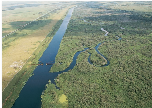
FIGURE 13.25 The naturally meandering Kissimmee River (right channel) was straightened by the Army Corps of Engineers (left) for flood control 30 years ago. Now the Corps is attempting to reverse its actions and restore the Kissimmee and its associated wetlands to their original state.
