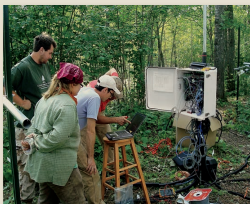
FIGURE 2.2 A student researcher adjusts the electrical panel that controls heat lamps and heating cables.
