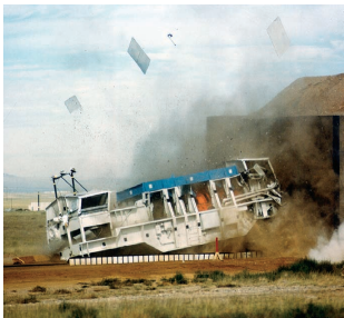
FIGURE 19.27 A test railcar carrying a spent nuclear fuel shipping cask slams into a concrete wall at 130 km/hr (81 mph). The cask survived without injury. Even so, many people don't want nuclear waste shipped through their city. Would you?
