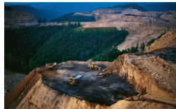
FIGURE 19.8 One of the most environmentally destructive methods of coal mining is mountaintop removal. Up to 100 m of the mountain is scraped off and pushed into the valley below, burying forests, streams, farms, cemeteries, and sometimes houses.
