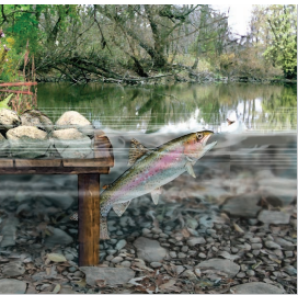
FIGURE 13.30 A lunker structure is a multilevel wooden framework that rests on the stream bottom and can be anchored to the shore. The top of the box is covered with rock, soil, and vegetation. Openings in the structure provide hiding places for fish.
