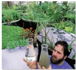
FIGURE 8.27 Bioreactors, such as these "living machines" from Ocean Arks International use living communities that mimic natural ecosystems to treat water. Polluted water (right flask) can be purified to drinking water quality (left flask).
