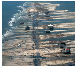
FIGURE 14.24 The aftermath of Hurricane Katrina on Dauphin Island, Alabama. Since 1970 this barrier island at the mouth of Mobile Bay has been overwashed at least five times. More than 20 million yd 3 (15 million m 3 ) of sand has been dredged or trucked in to restore the island. Some beach houses have been rebuilt, mostly at public expense, five times. Does it make sense to keep rebuilding in such an exposed place?
