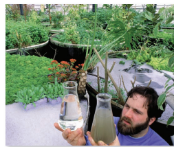
FIGURE 8.27 Bioreactors, such as these "living machines" from Ocean Arks International use living communities that mimic natural ecosystems to treat water. Polluted water (right flask) can be purified to drinking water quality (left flask).
