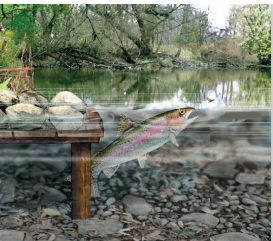
FIGURE 13.30 Aunker structure is a multilevel wooden framework that rests on the stream bottom and can be anchored to the shore. The top of the box is covered with rock, soil, and vegetation. Openings in the structure provide hiding places for fish.
