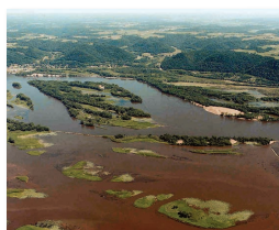
FIGURE 13.22 Dams on the upper Mississippi River have created a series of large lakes. Currents created by wind, floods, and river traffic keep the soft sediment stirred up so that wetland plants can't take root. To restore these backwaters, the Army Corps is experimenting with wing dams (see thin white lines between islands) that will allow the mud to solidify and turn into marshlands.
