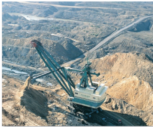
FIGURE 14.12 Some giant mining machines stand as tall as a 20-story building and can scoop up thousands of cubic meters of rock per hour.
