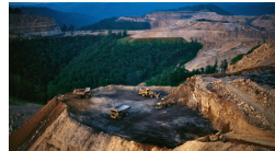
FIGURE 19.8 One of the most environmentally destructive methods of coal mining is mountaintop removal. Up to 100 m of the mountain is scraped off and pushed into the valley below, burying forests, streams, farms, cemeteries, and sometimes houses.
