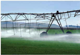
FIGURE 10.13 Downward-facing sprinklers on this center-pivot irrigation system deliver water more efficiently than upward-facing sprinklers.
