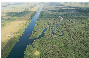
FIGURE 13.25 The naturally meandering Kissimmee River (right channel) was straightened by the Army Corps of Engineers (left) for flood control 30 years ago. Now the Corps is attempting to reverse its actions and restore the Kissimmee and its associated wetlands to their original state.
