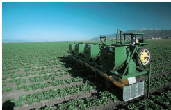
FIGURE 10.30 This machine, nicknamed the "sabad vac," sucks bugs off crops as an alternative to treating them with toxic chemicals.
