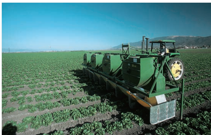
FIGURE 10.30 This machine, nicknamed the “salad vac,” vacuums bugs off crops as an alternative to treating them with toxic chemicals.
