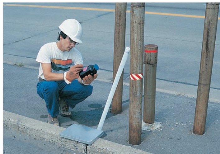
FIGURE 25.4 Many interesting, well-paying jobs are opening up in environmental fields. Here an environmental technician takes a sample from a monitoring well for chemical analysis.
