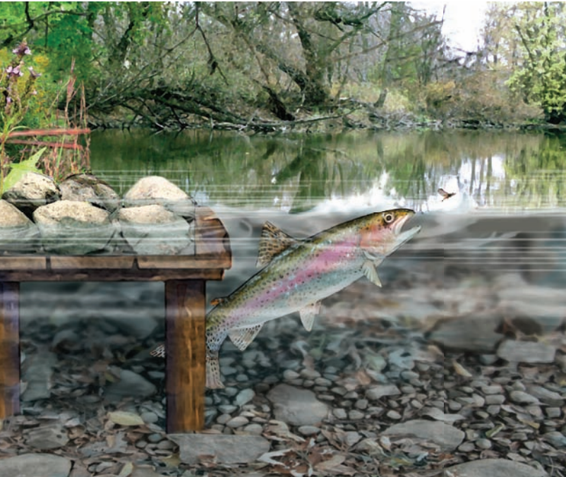
FIGURE 13.30 A lunker structure is a multilevel wooden framework that rests on the stream bottom and can be anchored to the shore. The top of the box is covered with rock, soil, and vegetation. Openings in the structure provide hiding places for fish.
