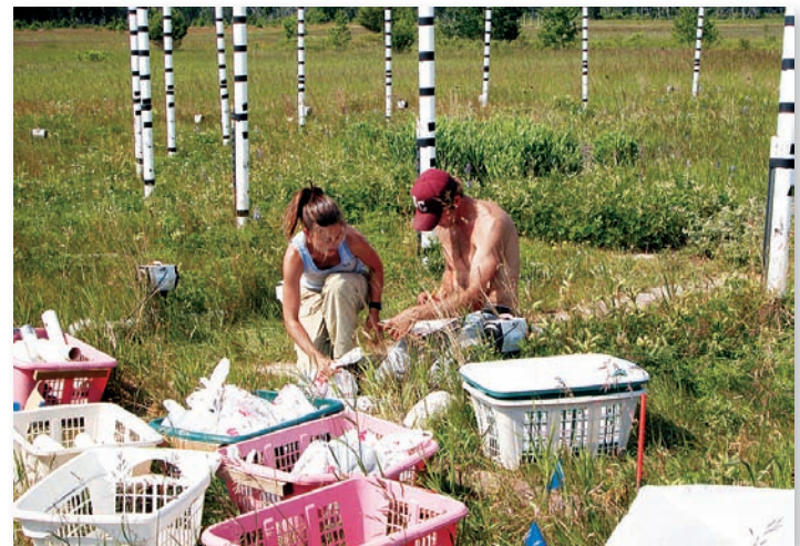
FIGURE 2.10 Environmental scientists often study open systems. Here students at Cedar Creek study the climate-vegetation system, gathering plant samples that grew in carbon dioxide-enriched air pumped from the white poles, but other factors (soil, moisture, sunshine, temperature) are not controlled.
