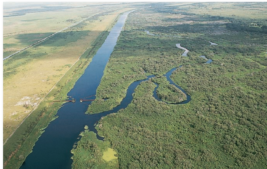
FIGURE 13.25 The naturally meandering Kissimmee River (right channel) was straightened by the Army Corps of Engineers (left) for flood control 30 years ago. Now the Corps is attempting to reverse its actions and restore the Kissimmee and its associated wetlands to their original state.
