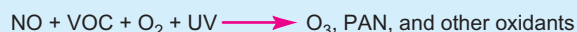
FIGURE 16.7 Secondary production of urban smog oxidants by photochemical reactions in the atmosphere.
