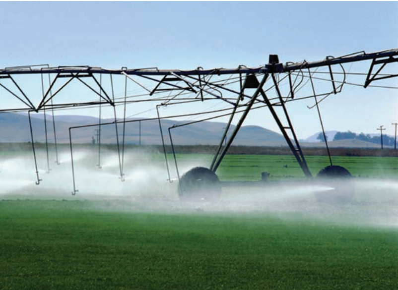
FIGURE 10.13 Downward-facing sprinklers on this center-pivot irrigation system deliver water more efficiently than upward-facing sprinklers.
