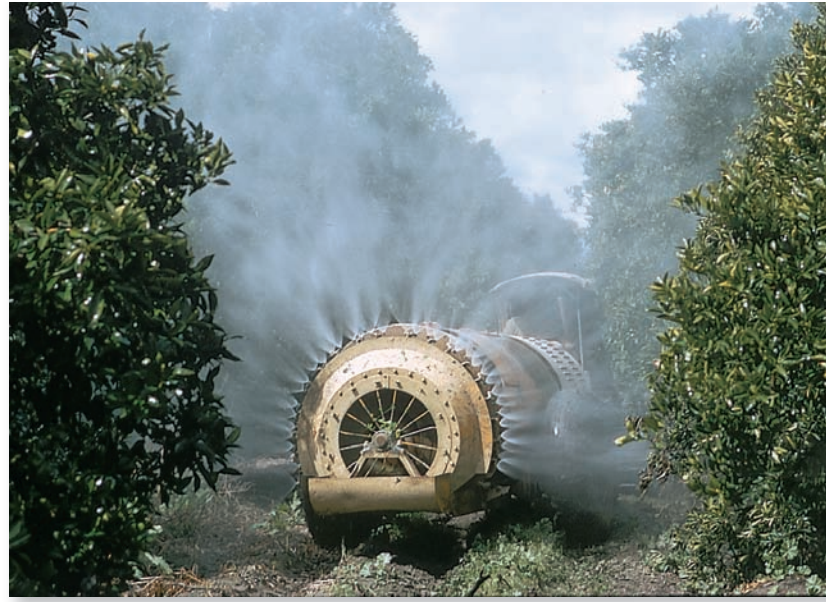
FIGURE 10.22 This machine sprays insecticide on orchard trees—and everything nearby. Up to 90 percent of pesticides applied in this fashion never reach target organisms.
