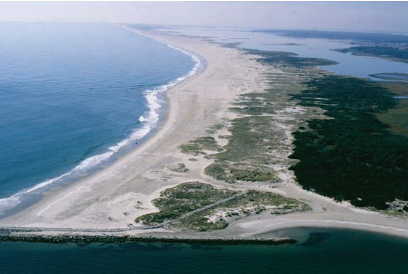
FIGURE 5.18 A barrier island, Assateague, along the Maryland–Virginia coast. Grasses cover and protect dunes, which keep ocean waves from disturbing the bay, salt marshes, and coast at right. Roads cut through the dunes expose them to erosion.
