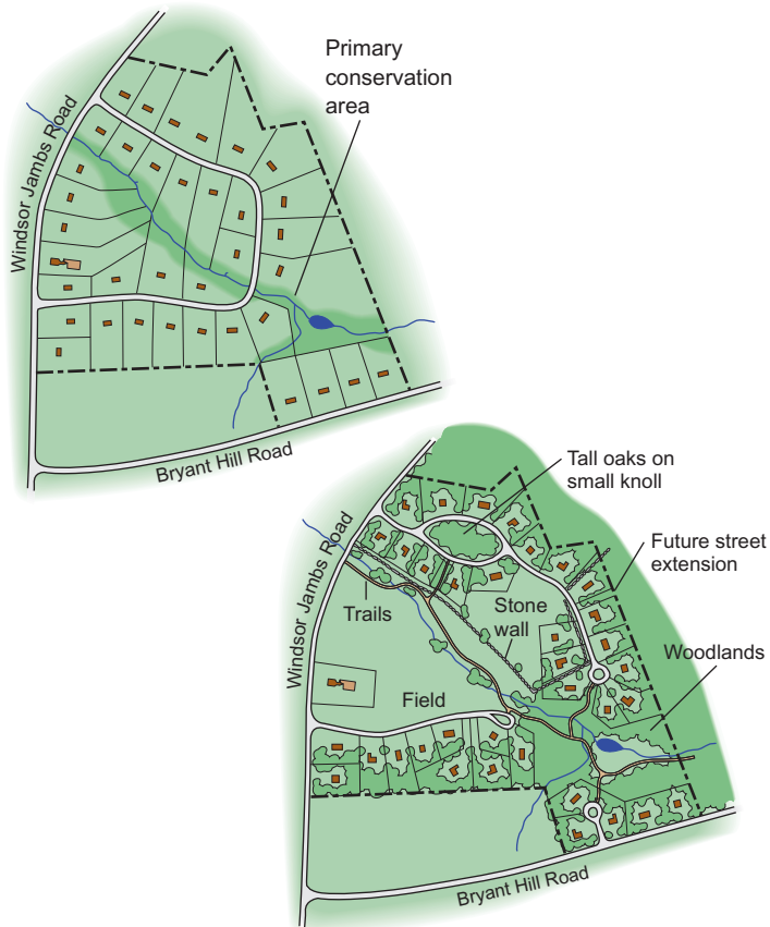
FIGURE 22.21 Conventional subdivision ( top ) and an open space plan ( bottom ). Although both plans provide 36 home sites, the conventional development allows for no public space. Cluster housing on smaller lots in the open space design preserves at least half the area as woods, prairie, wetlands, farms, or other conservation lands, while providing residents with more attractive vistas and recreational opportunities than a checkerboard development.
