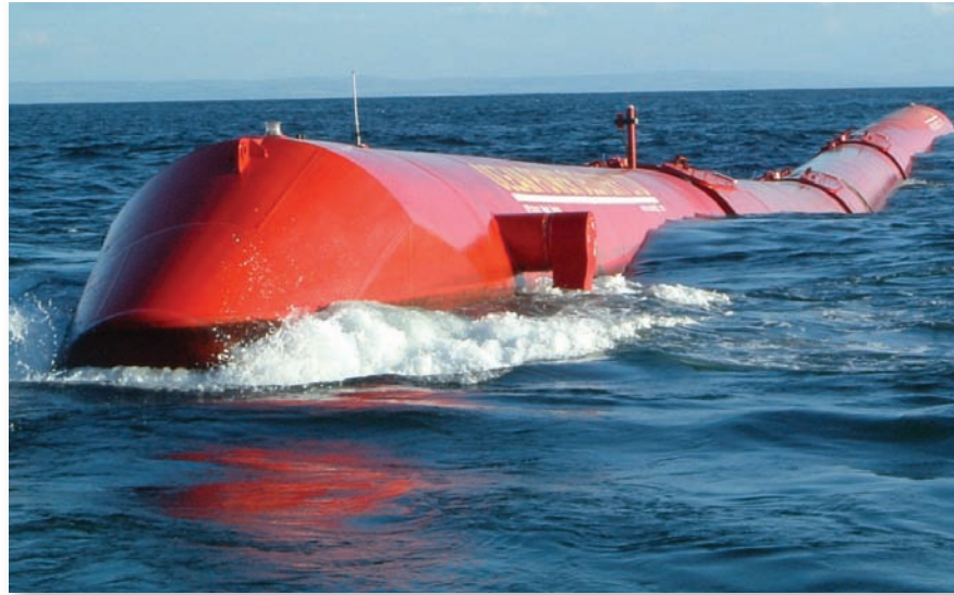
FIGURE 20.33 The Pelamis wave converter (named after a sea snake) is a 125 m long and 3.5 m diameter tube-hinged, so it undulates as ocean swells pass along it. This motion drives pistons that turn electrical generators. Energy experts calculate that capturing just 1 to 2 percent of global wave power could supply at least 16 percent of the world's electrical demand.
