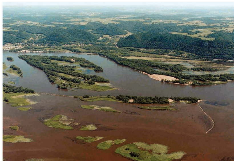
FIGURE 13.22 Dams on the upper Mississippi River have created a series of large lakes. Currents created by wind, floods, and river traffic keep the soft sediment stirred up so that wetland plants can’t take root. To restore these backwaters, the Army Corps is experimenting with wing dams (see thin white lines between islands) that will allow the mud to solidify and turn into marshlands.
